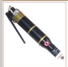
Pneumatic depaneling tool. The DPP is suitable for the quick, economic and secure separation of PCBs, leaving the cut edges well finished. The interchangeability of the blades, made from special steel in various thicknesses, enable it to satisfy all customer requirements. (Isthmus lenght 1÷3 mm)
