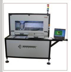
DPA1000 is an automatic depaneling system. Using a vertical milling cutter this system allows to cut isthmus in any direction, following linear or circular lines. DPA1000 functioning is performed by a Personal Computer which manages:
