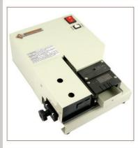
2000 SE is an electric machine for the forming and cutting(standard height 3mm) of untaped electronic component terminals.
