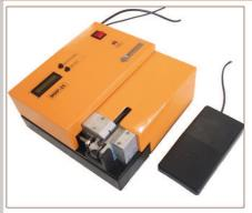
The MMP25 is an electric machine, CE approved, designed for the crimping of several STOCKO terminals
