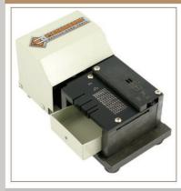
2000S is a pneumatic machine for the forming and cutting(standard height 3mm) of untaped electronic component terminals.
