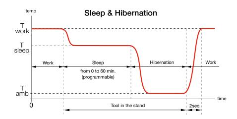
Tip life increases exponentially by using lower temperatures as shown. Using the **Sleep** mode the temperature is further reduced, which extends tip life by 5.
